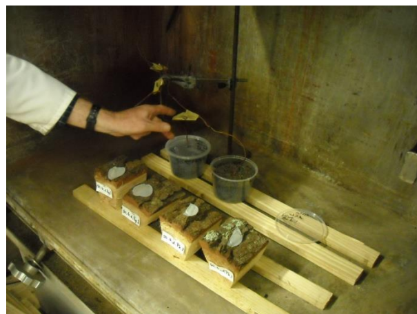
Fig. 9: Exposed micromesh on wood and pottles containing soil for heat treatments
