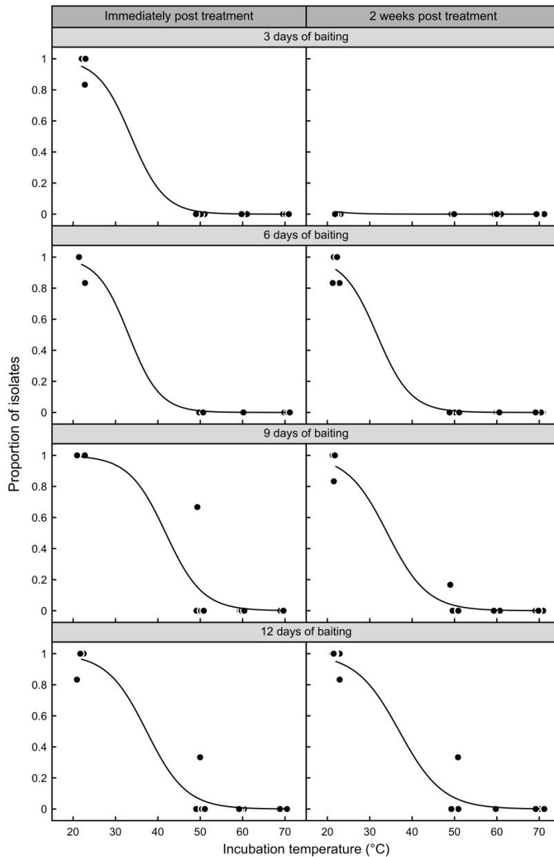
Figure 5: Proportion of *Phytophthora* taxon *Agathis* oospore isolates recovered by baiting 3, 6, 9 and 12 days post treatment at 22, 50, 60 and 70°C. Analysis was carried out on fresh samples (Immediately post treatment) and on a second set of samples stored at room temperature for two weeks prior to analysis (2 weeks post treatment). Solid lines represent predicted values from a binomial generalized linear mixed effects model,  $n = 10$ .
