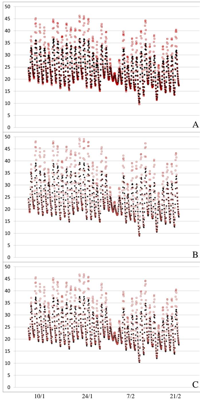
**Figure 10: Temperature of solarization bags measured hourly between 13 January and 20 February 2015 with black (■) and clear (□) surfaces facing up when laid on (A) cement, (B) polystyrene and (C) ground.**
