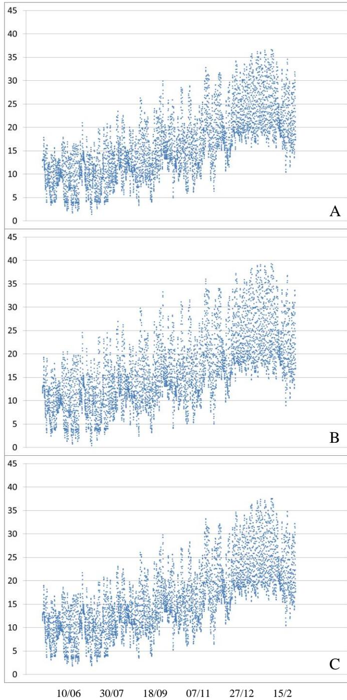
**Figure 9: Temperature of solarization bags measured hourly between 6 June 2014 and 20 February 2015 with the black surface of the bag facing up when laid on (A) cement, (B) polystyrene and (C) ground.**
