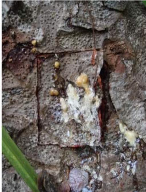
**Figure 12** Lesion sample delimited by chiselling around edge.
