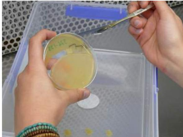
**Figure 7** Oblong blocks (1.5 × 1 cm) of V8 juice agar from the advancing colony being placed into 7-L ‘Klip It’ bioassay vessel.
