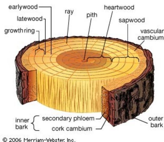
**Figure 2** Cross section schematic of the generic anatomical layers present within tree stems (source: Britannica.com)
