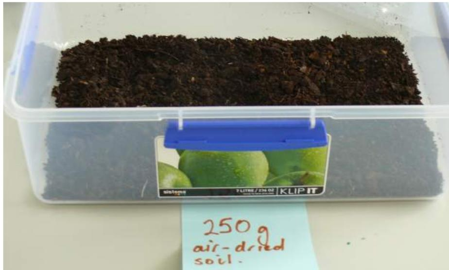
**Figure 10** Soil-based bioassay in 7-L 'Klip It' container.
