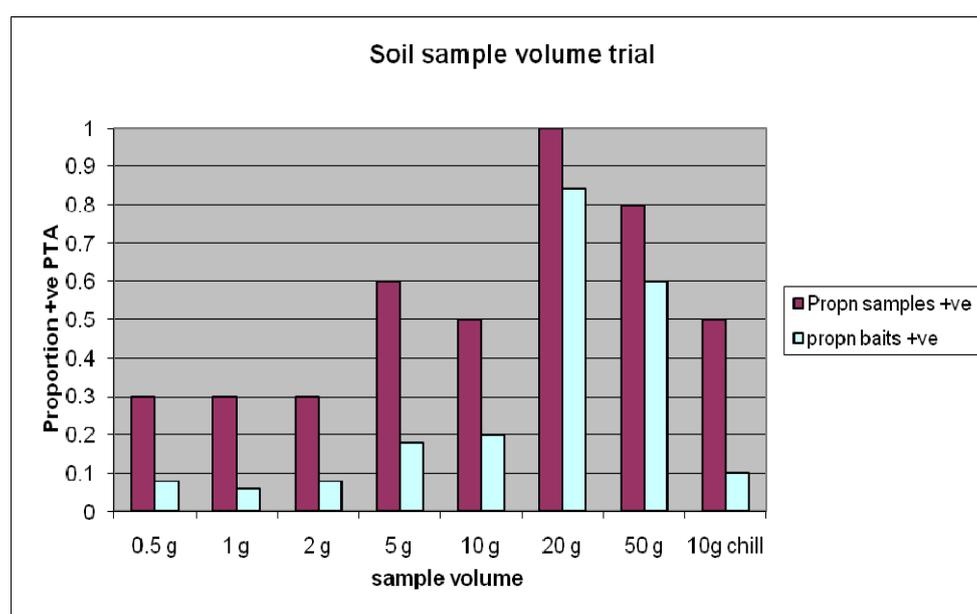
**Figure 16** Comparative PTA recoveries from a range of seven soil-sample sizes (graph includes 10-g soil samples assayed with chilled RO water).
